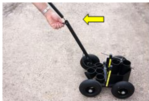
Assemble handle and fasten with screw.
